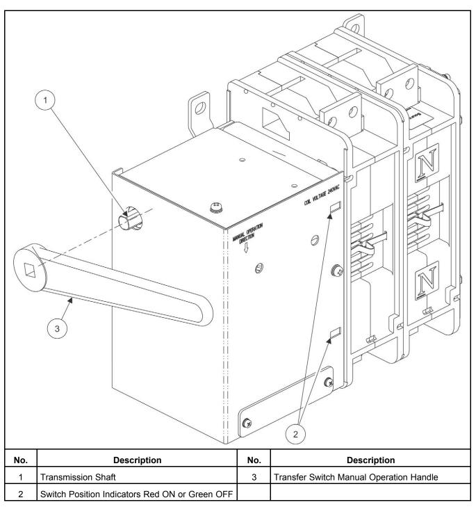
FIGURE 32. RA412N3 AND RA412S3 MANUAL OPERATION HANDLE
