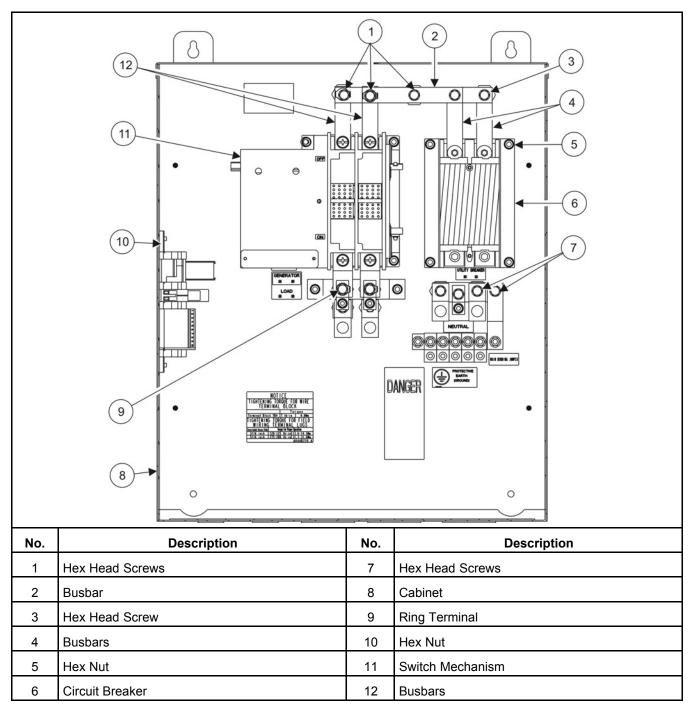
FIGURE 26. INTERIOR COMPONENTS FOR RA112S3 AND RA212S3 SERVICE ENTRANCE MODELS (SPEC A)
