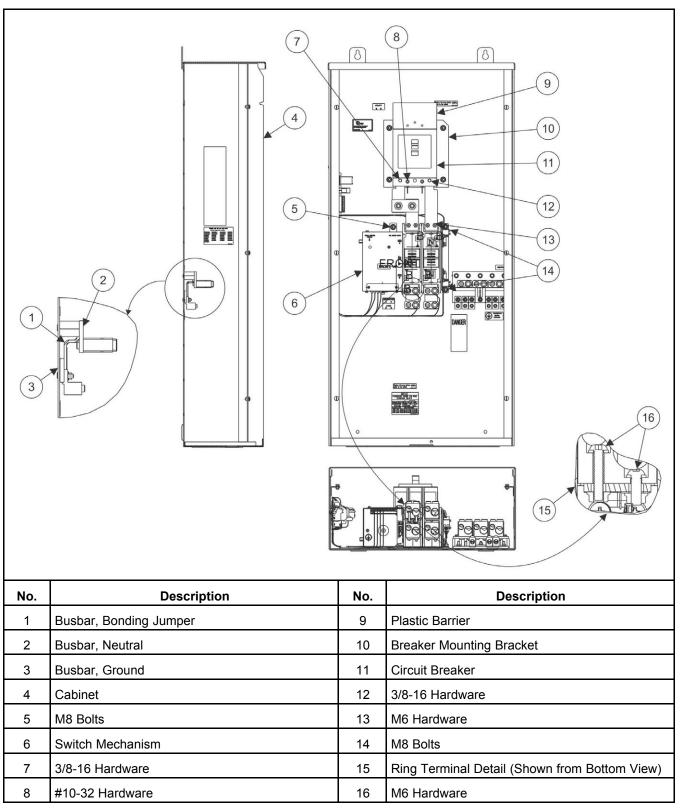
FIGURE 28. INTERIOR COMPONENTS FOR RA412S3 SERVICE ENTRANCE MODELS
