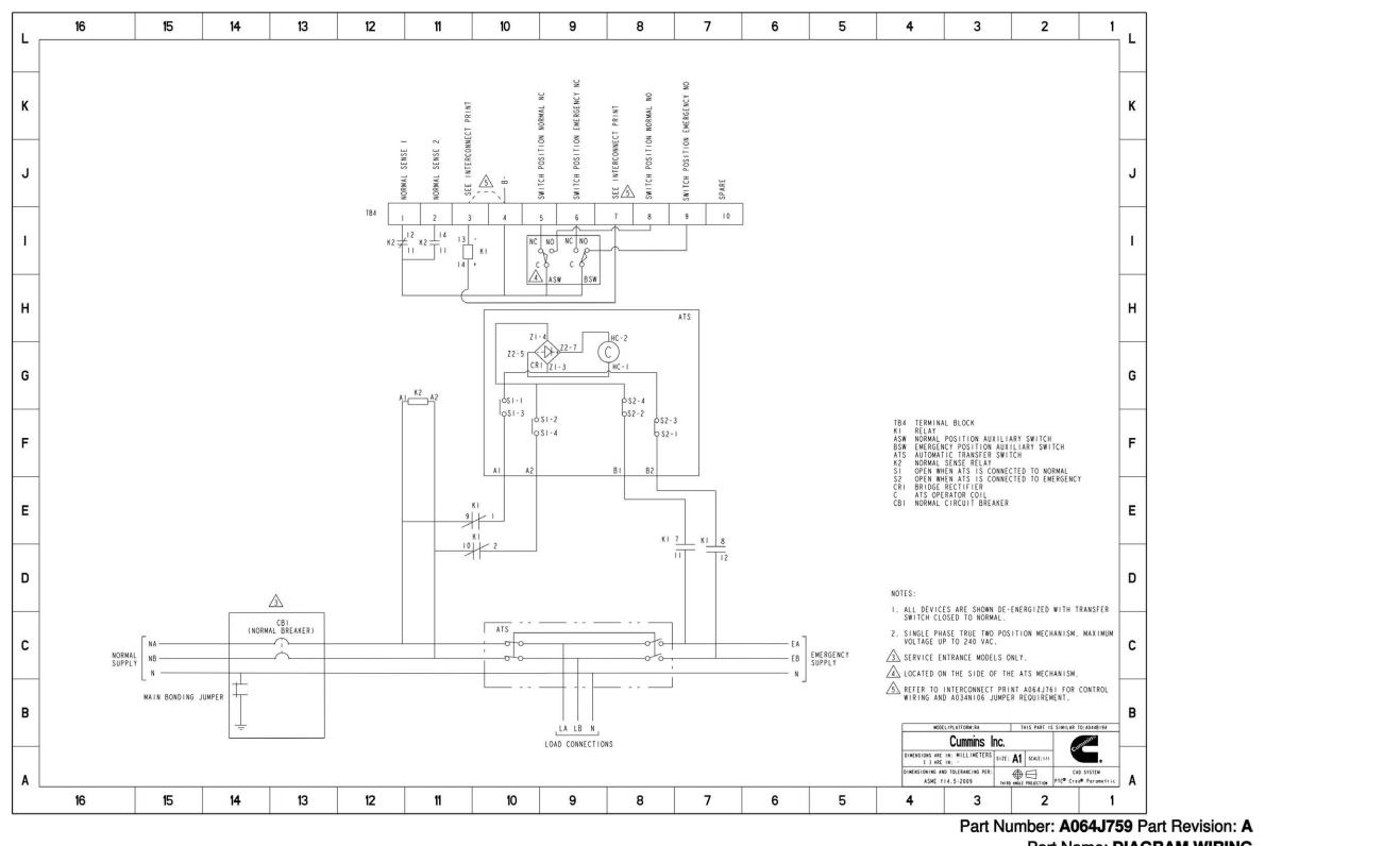
FIGURE 46. RA112N3, RA212N3, RA112S3, AND RA212S3 TRANSFER SWITCH WIRING DIAGRAM (SHEET 1 OF 2) (SPEC B)
