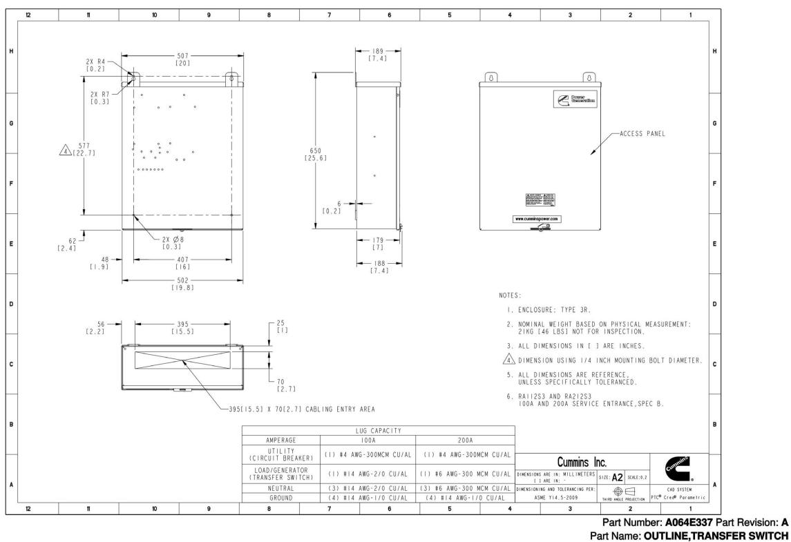
FIGURE 63. RA112S3 AND RA212S3 CONTROL BOX OUTLINE DRAWING (SPEC B)
