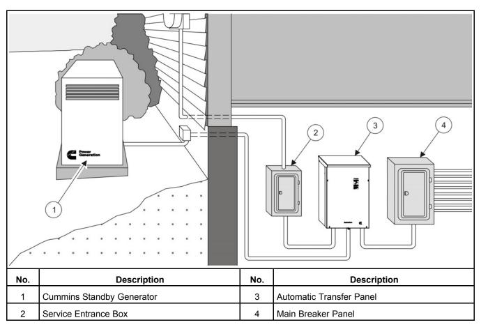
FIGURE 20. TYPICAL WALL-MOUNT INSTALLATION OF NON-SERVICE ENTRANCE MODELS
