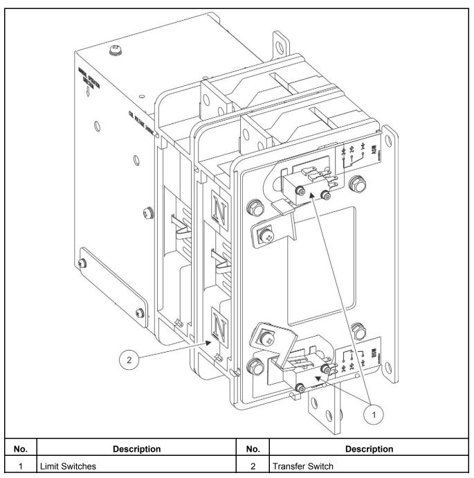
FIGURE 30. RA412N3 AND RA412S3 TRANSFER SWITCH REMOVAL
