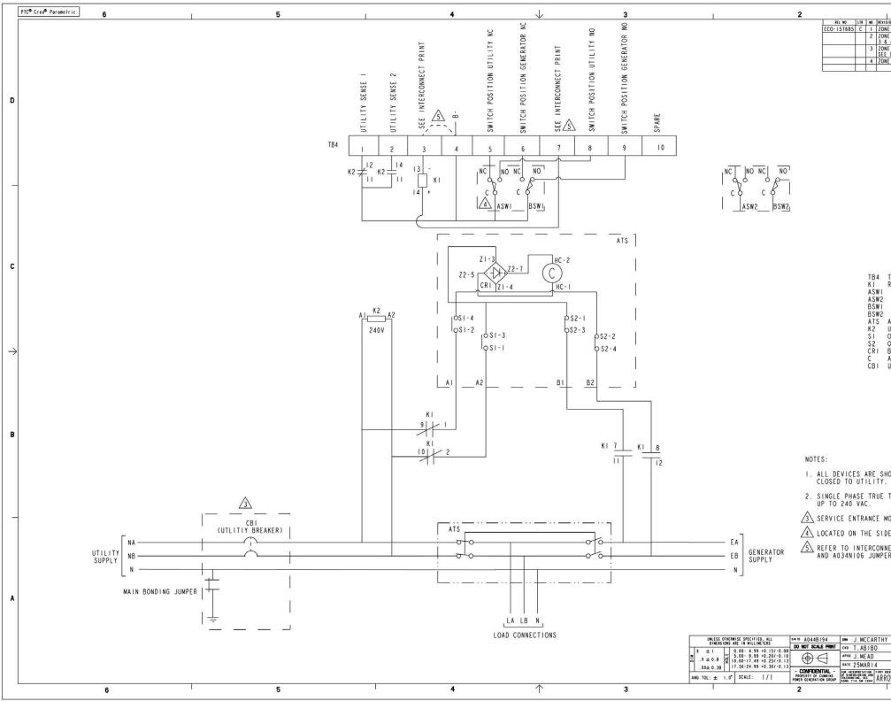
FIGURE 48. RA412N3 AND RA412S3 TRANSFER SWITCH WIRING DIAGRAM (SHEET 1 OF 2)
