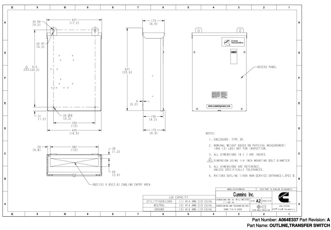
FIGURE 59. RA112N3 CONTROL BOX OUTLINE DRAWING (SPEC B)
