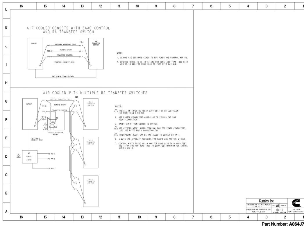
FIGURE 55. RA112N3, RA212N3, RA112S3, AND RA212S3 TRANSFER SWITCH INTERCONNECTIONS (SHEET 3 OF 3) (SPEC B)
