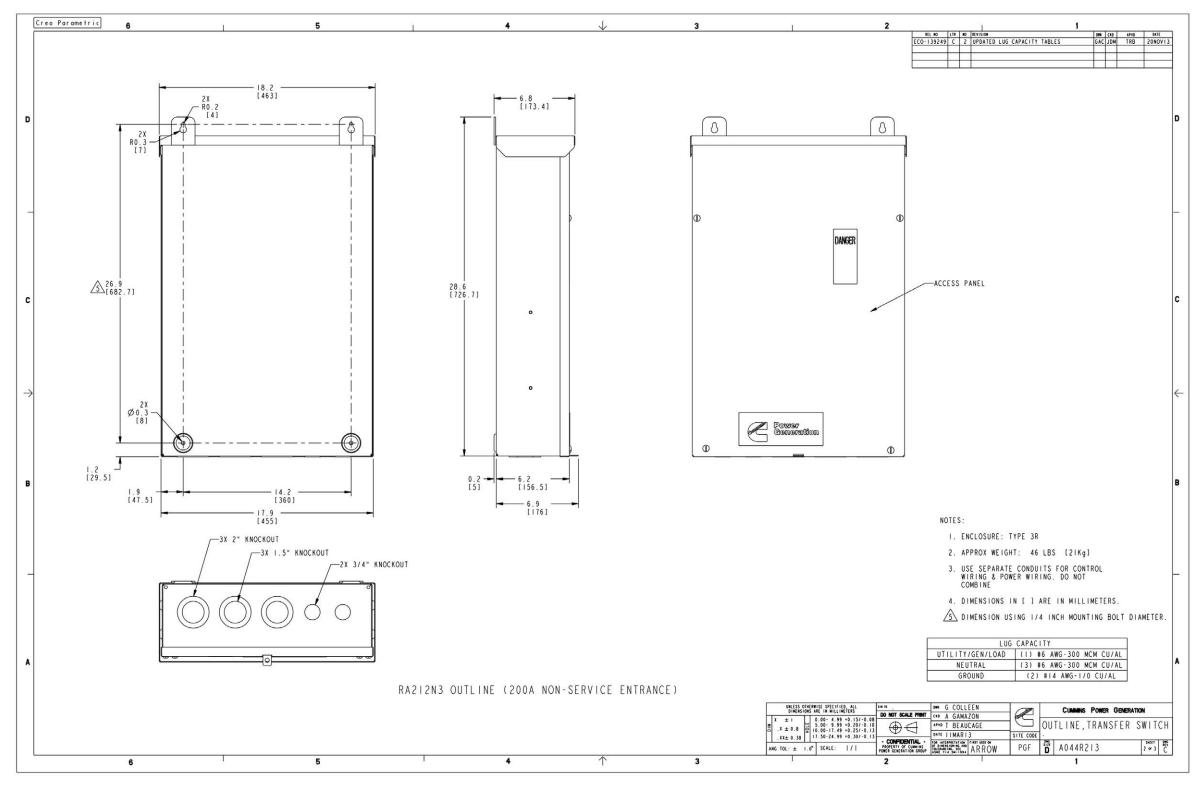
FIGURE 60. RA212N3 CONTROL BOX OUTLINE DRAWING (SPEC A)
