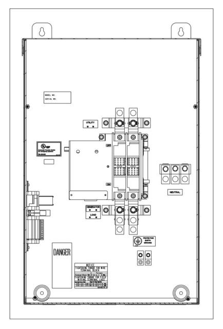
FIGURE 1. RA112N3 AND RA212N3 NON-SERVICE ENTRANCE TRANSFER SWITCH (WITH DOOR PANEL REMOVED) (SPEC A-B)
