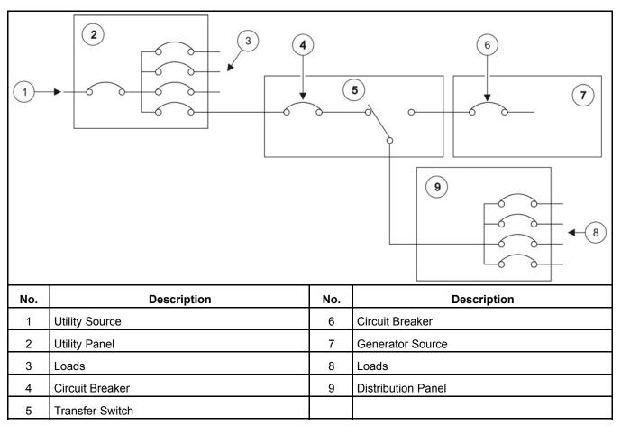
FIGURE 18. PARTIAL COVERAGE SYSTEM (SERVICE ENTRANCE MODEL)
