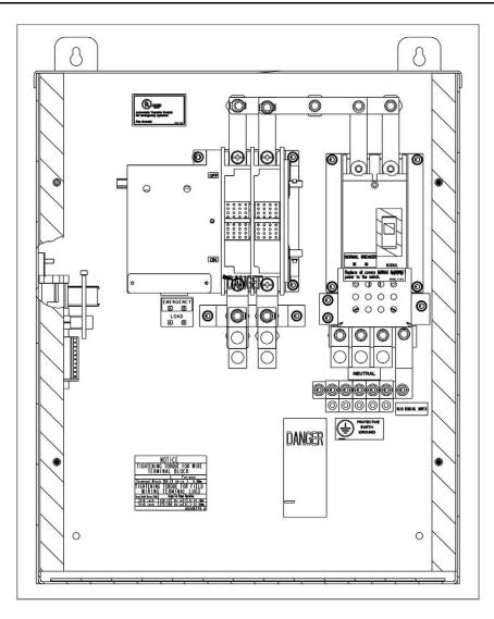
FIGURE 4. RA112S3 AND RA212S3 SERVICE ENTRANCE TRANSFER SWITCH (WITH DOOR PANEL REMOVED) (SPEC B)
