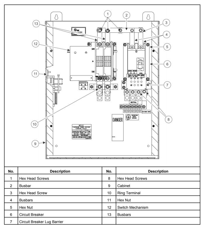
FIGURE 27. INTERIOR COMPONENTS FOR RA112S3 AND RA212S3 SERVICE ENTRANCE MODELS (SPEC B)
