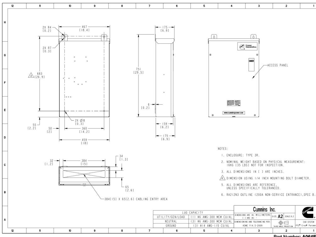
FIGURE 61. RA212N3 CONTROL BOX OUTLINE DRAWING (SPEC B)
