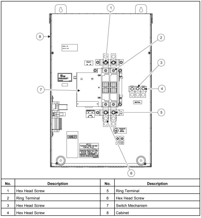
FIGURE 24. INTERIOR COMPONENTS FOR RA112N3 AND RA212N3 NON-SERVICE ENTRANCE MODELS (SPEC A-B)
