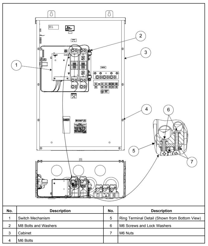
FIGURE 25. INTERIOR COMPONENTS FOR RA412N3 NON-SERVICE ENTRANCE MODELS
