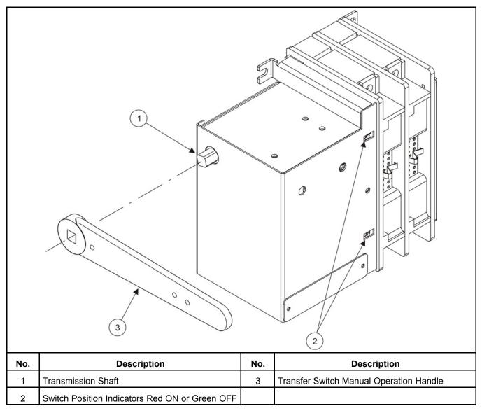
FIGURE 31. RA112N3, RA212N3, RA112S3, AND RA212S3 MANUAL OPERATION HANDLE
