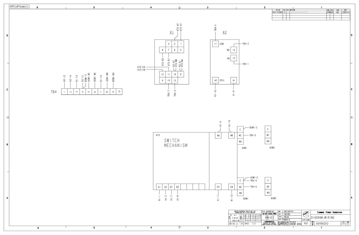
FIGURE 49. RA412N3 AND RA412S3 TRANSFER SWITCH WIRING DIAGRAM (SHEET 2 OF 2)
