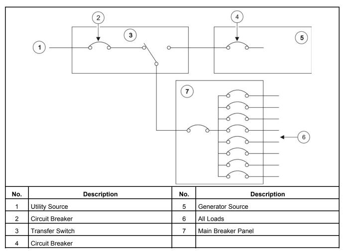
FIGURE 21. TOTAL COVERAGE SYSTEM (SERVICE ENTRANCE MODEL)
