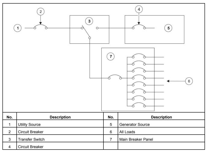
FIGURE 19. TOTAL COVERAGE SYSTEM (NON-SERVICE ENTRANCE MODEL)
