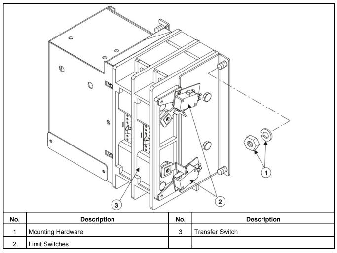
FIGURE 29. RA112N3, RA212N3, RA112S3, AND RA212S3 TRANSFER SWITCH REMOVAL
