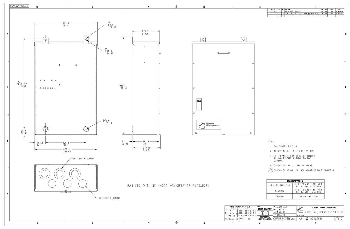
FIGURE 64. RA412N3 CONTROL BOX OUTLINE DRAWING
